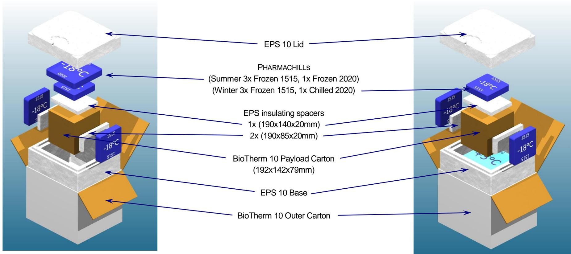
Chilled PHARMACHILLS should be conditioned at +5°C for a minimum of 24 hours before use. Frozen PHARMACHILLS should be conditioned at -18°C for a minimum of 24 hours and then for approximately 20 minutes at factory ambient +20°C (± 5) before system assembly.
