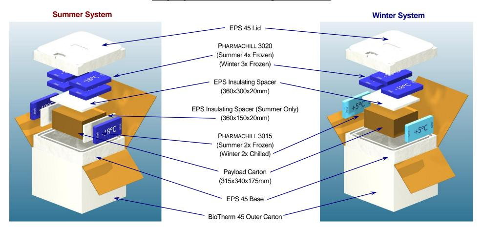
Chilled Pharmachill s should be conditioned at +5°C for a minimum of 24 hours before use. Frozen Pharmachill s should be conditioned at -18°C for a minimum of 24 hours and then for approximately 20 minutes at factory ambient +20°C (± 5) before system assembly.
