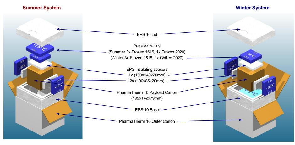
Chilled PHARMACHILLs should be conditioned at +5°C for a minimum of 24 hours before use. Frozen PHARMACHILLs should be conditioned at -18°C for a minimum of 24 hours and then for approximately 20 minutes at factory ambient +20°C (± 5) before system assembly.
