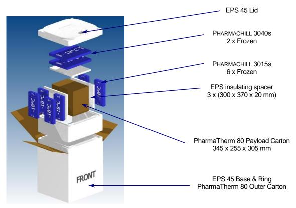
Chilled Pharmachills should be conditioned at +5°C for a minimum of 24 hours before use. Frozen Pharmachills should be conditioned at -18°C for a minimum of 24 hours and then for approximately 20 minutes at factory ambient +20°C (± 5) before system assembly.
