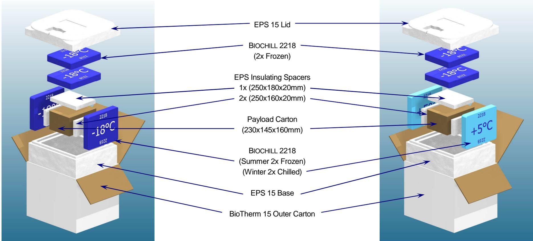
Chilled BIOCHILLS should be conditioned at +5°C for a minimum of 24 hours before use. Frozen BIOCHILLS should be conditioned at -18°C for a minimum of 24 hours and then for approximately 20 to 30 minutes at factory ambient +20°C (± 5) before system assembly.
