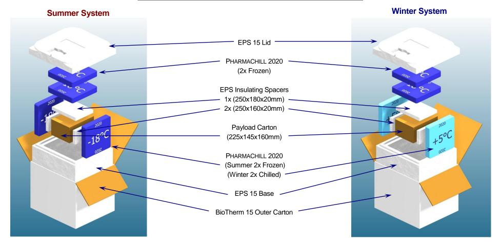
Chilled Pharmachills should be conditioned at +5°C for a minimum of 24 hours before use. Frozen Pharmachills should be conditioned at -18°C for a minimum of 24 hours and then for approximately 20 to 30 minutes at factory ambient +20°C (± 5) before system assembly.
