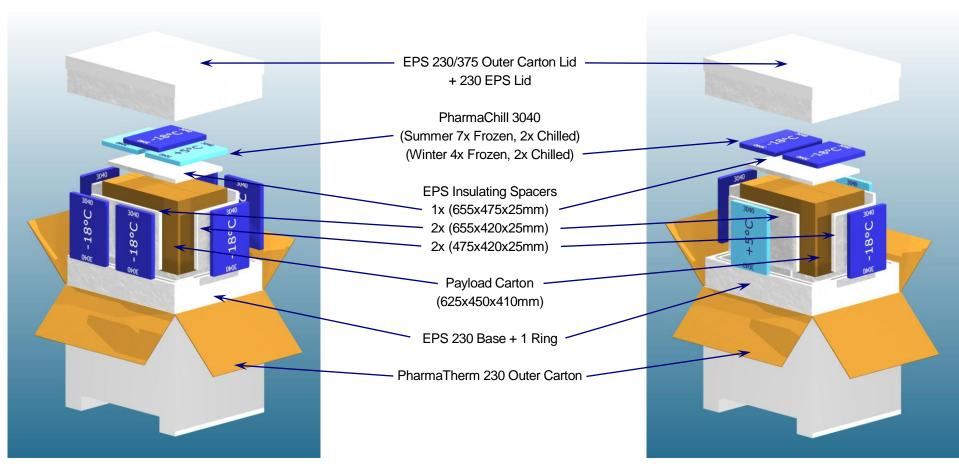
Chilled PharmaChills should be conditioned at +5°C for a minimum of 24 hours before use. Frozen PharmaChills should be conditioned at -18°C for a minimum of 24 hours and then for between 20 to 30 minutes at factory ambient +20°C (± 5) before system assembly.
